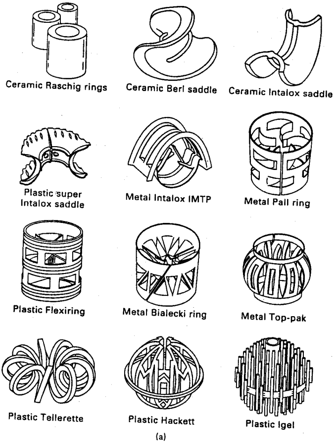
(a) Figure 6.7 Typical materials used in a packed column: (a) random packing materials; (continued)
